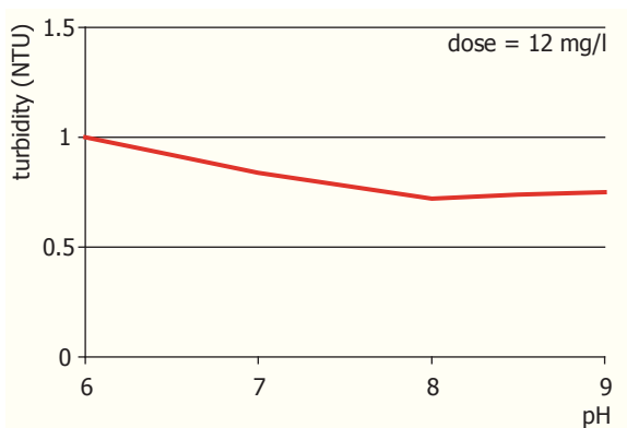
Figure 12 - Results of jar test experiment with varying pH
